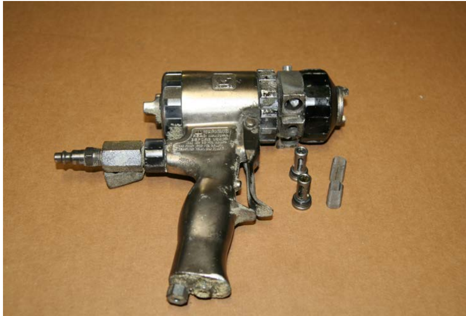
Graco Fusion AP Gun. Remove and leave out gun screens.
